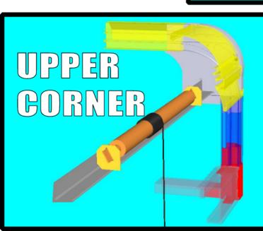
Realignment of counterbalance cable to door panel makes our roll-up door easier to operate.
