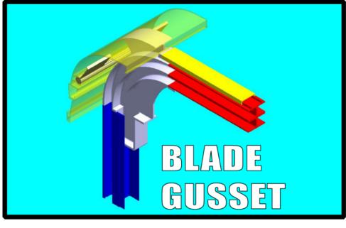
All-aluminum corner and intermediate machined castings are "sleeve fitted" to rub rail, door tracks and door post to form a positive, stress-free connection to enhance strength and durability of the total unit.
