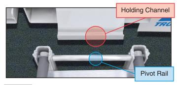
STEP 2 Align pivot rail with holding channel.
