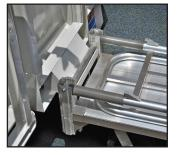
STEP 4 Push Mickey's Route Buddy forward so pivot rail slides over and into the holding channel with no lifting.
