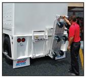
STEP 5 Pivot rail tightly holds Mickey's Route Buddy within the holding channel so it's ready to be locked in place.
