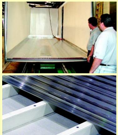
Floor is attached to 2.50" composite isolators to accommodate 3.50" of urethane insulation. Mickey's Thermal Bear body features flat walls inside and out. A smooth interior lining of .090 glass board has a built-in 6" aluminum scuff liner at floor level to protect the surface during loading and unloading. There are no exposed fasteners inside the body to damage your products.
