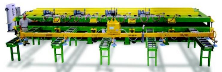
Mickey uses a unique automated "platen process" rather than the conventional "hand shoring" manual technique which is more time consuming and much less accurate due to human error. The automated platen process heats insulation cavities to a perfect 100 degrees so that foam reaches optimum density. The process eliminates over pouring and reduces waste, while eliminating insulation voids.
