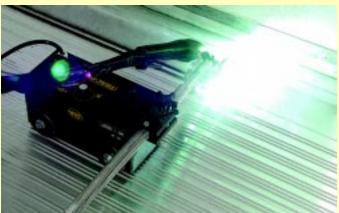
Aluminum floor sections are fully welded with an automated process insuring each seam is water tight.
