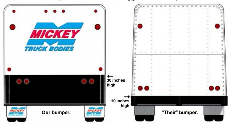
The standard beverage trailer bumper these days is 10 inches high. The Mickey bumper is a full 30 inches high, and that difference goes a long way in preventing costly override damage to your trailer.
